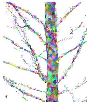
Fig. 1. TLS-point cloud partitioned into surface patches.
