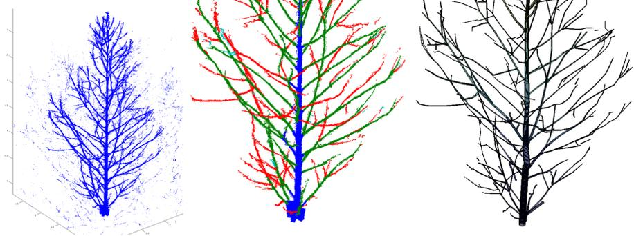
Fig. 2. Example of the 3D architecture of the top part of an Eucalyptus tree. Left, raw point cloud; middle, segmented point cloud; and right, reconstructed cylinder model.
