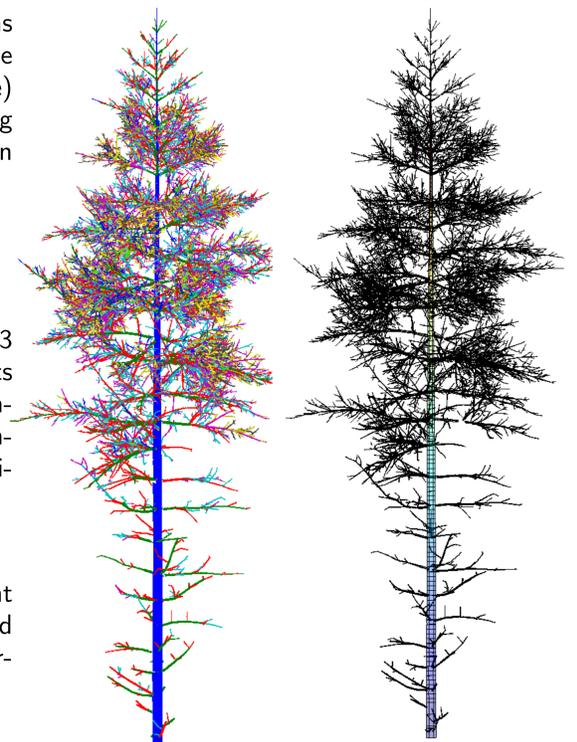
Fig. 3. The segmented point cloud (left) and reconstructed cylinder model (right) of the artificial Scots pine.
