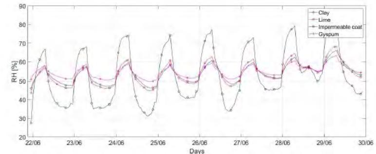
RH variation in a simulated room with different wall finishes.
