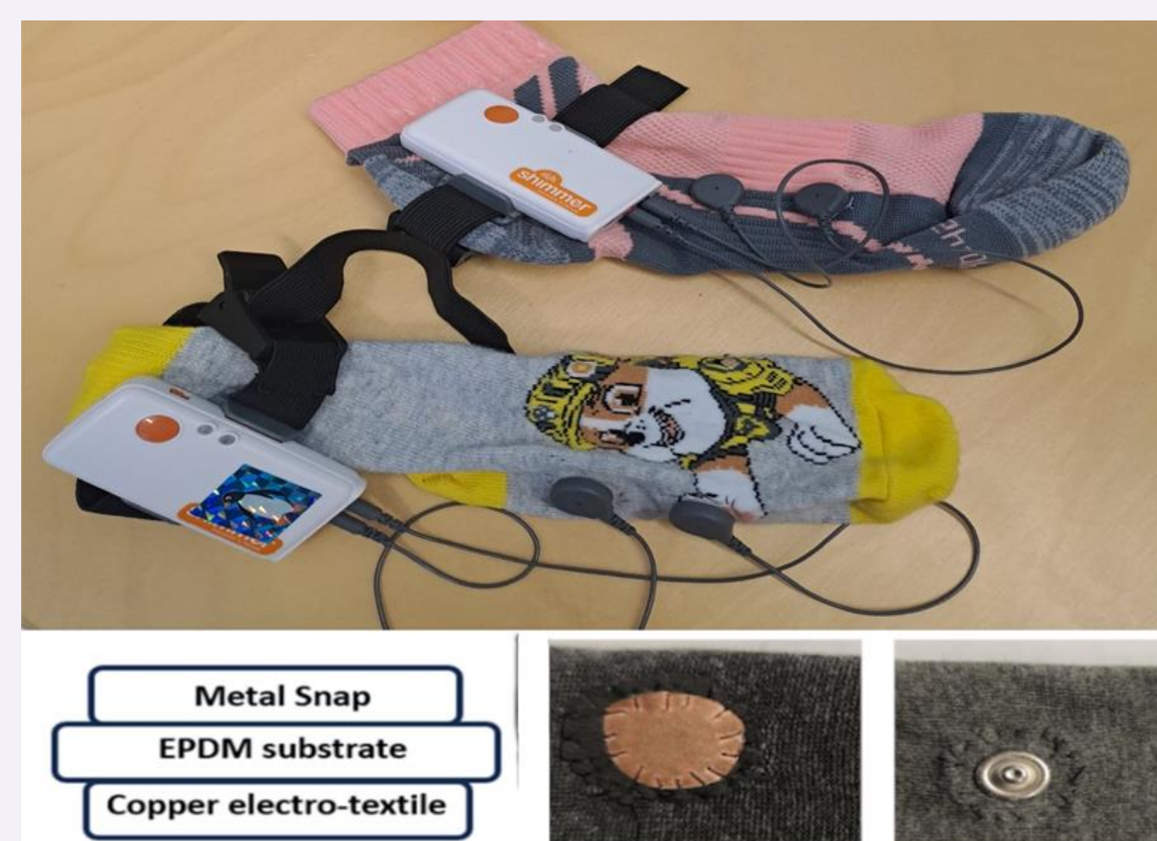
Fig 1. EDA was measured using a Shimmer3 GSR+ device connected via textile electrodes embedded in a soft sock. The electrodes were constructed from copper based electro textile (thickness 0.08 mm; surface resistance < 0.05 ohm/square; 35% copper per 880 g/m 2 ), (modified from Rahman, et al., 2024)
