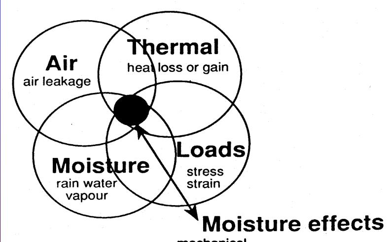
biological (rot) physical (dimensions) chemical (corrosion) mechanical freeze-thaw crackpropagation
