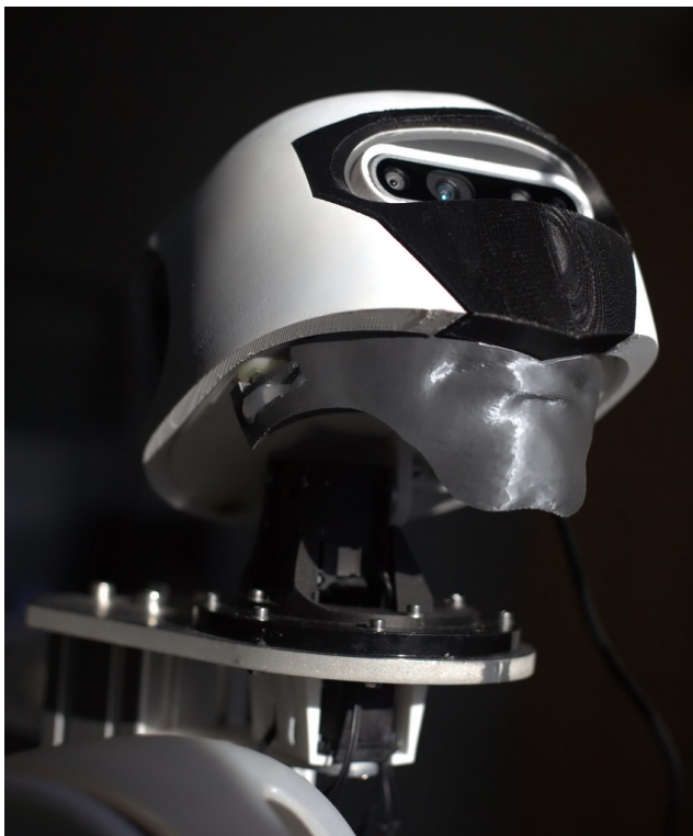
Fig. 6. Resulting design of aesthetic facade demonstrating a bionic look through 3D scanned data and its manipulation.
