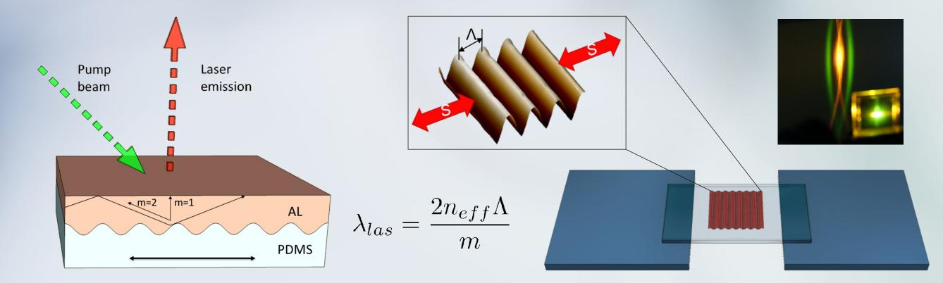
**Operating principle.** DFB laser have a periodically structured active layer. The emission wavelength is directly proportional to the corrugation period and can be selected by satisfying the Bragg condition. Actuation of LCE is used to tune the wavelength continuously.
