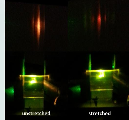
**Mechanical tuning.** The limits of tunability are explored by stretching a laser membrane mechanically. Stretching the membrane proved the spectral emission tuning over the whole gain region of the used laser dyes. A maximal tuning range of 77 nm was achieved using DCM2 laser dye in a Poly(vinyl acetate) matrix.<sup>2</sup>
