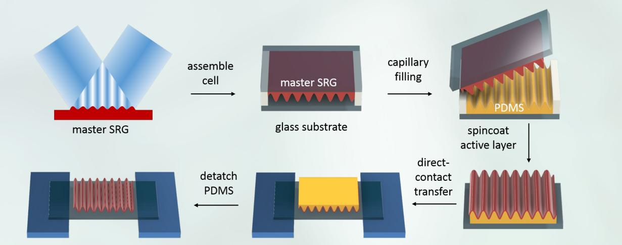
**Assembling.** The SRG is replicated into a thin layer of silicone. A solution containing a laser dye and a polymer is spincoated on the replica to create the laser membrane. A contact transfer method is used to translate the membrane from the silicone substrate onto the LCE actuator or any other support.
