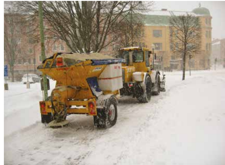
Figures 7 and 8. The prioritised cycle path network is maintained using a method that combines sweeping and salting. During heavy snowfall, ploughing is used instead of sweeping.
