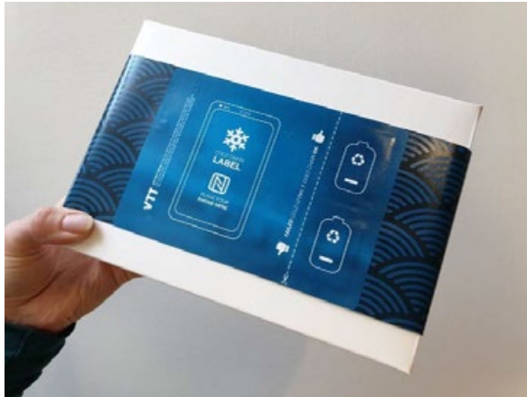
Figure 1. Rough design for temperature monitoring package.
