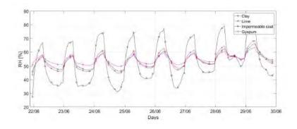
RH variation in a simulated room with different wall finishes.
