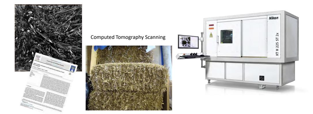
"Optimising orientation of the straw fibres in bales has successfully reduced thermal conductivity, compared to conventional agricultural bales, by 38%"
