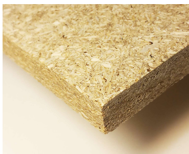
Porous board, 20 mm, 400 kg/m 3
