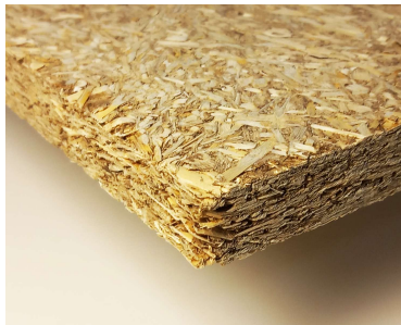
Porous board, 20 mm, 500 kg/m 3
