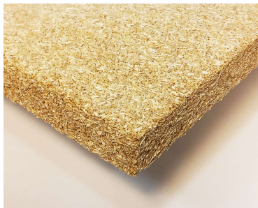
Porous board, 25 mm, 270 kg/m 3
