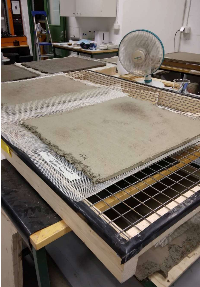
The board was dried in a stream of air and the surface of the plate was painted with clay starch paint
