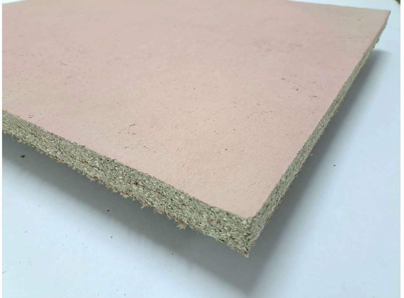
The board was dried in a stream of air and the surface of the plate was painted with clay starch paint
